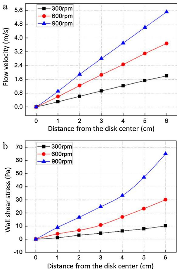
Fig. 3. Flow velocity (a) and wall shear stress (b) versus distance away from the rotation center under different rotation speeds of the disk.
