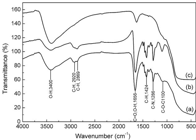
**Fig. 5** FTIRs spectra of (a) the as-sprayed TiO<sub>2</sub> hollow microspheres, (b) the as-sprayed TiO<sub>2</sub>-Fe<sub>3</sub>O<sub>4</sub> hollow microspheres, and (c) the post-spray calcined TiO<sub>2</sub>-Fe<sub>3</sub>O<sub>4</sub> hollow microspheres
