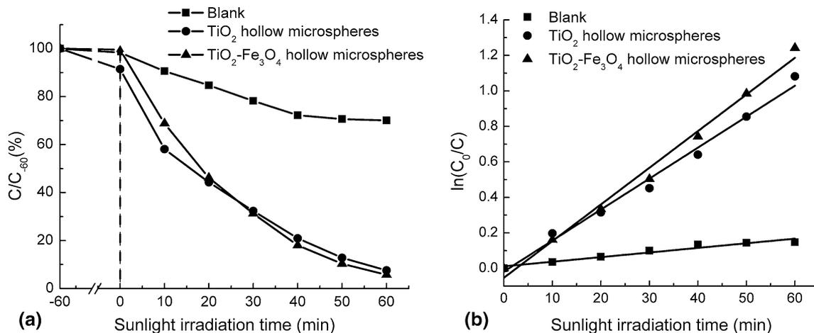
**Fig. 6** Photocatalytic activity assessment of the powder samples under sunlight irradiation, (a) variation of MB concentration vs. sunlight illumination time, and (b)  $\ln(C_0/C)$  against sunlight irradiation time in the presence or absence of the hollow microspheres
