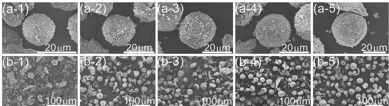
**Fig. 1** Typical SEM images showing the effect of spray power (a) and content of PVP in the starting suspension (b) on the sizes and the morphology of the hollow spheres, (a-1) net energy of 14 kW, (a-2) net energy of 20 kW, (a-3) net energy of 25 kW, (a-4) net energy of 30 kW, (a-5) net energy of 36 kW; (b-1) PVP content of 0.25%, (b-2) PVP content of 0.5%, (b-3) PVP content of 1.0%, (b-4) PVP content of 1.5%, (b-5) PVP content of 2.0%
