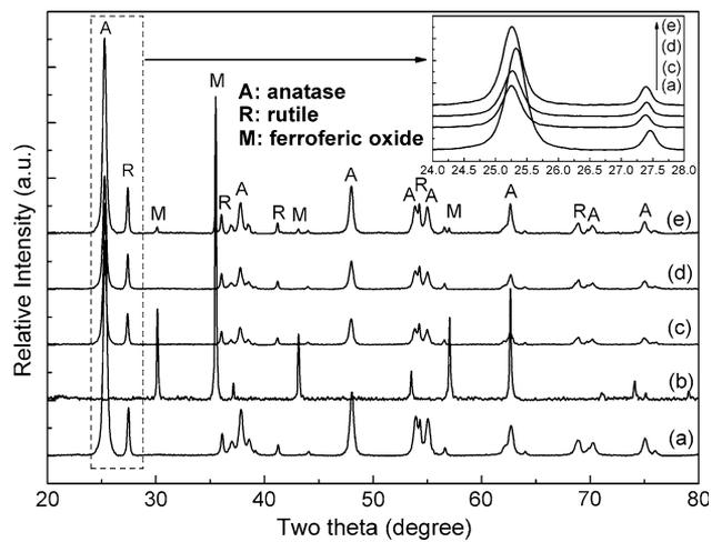
**Fig. 3** XRD patterns of (a) the starting P25 nano powder, (b) the starting  $\text{Fe}_3\text{O}_4$  nano powder, (c) the as-sprayed  $\text{TiO}_2$  hollow spheres, (d) the post-spray calcined  $\text{TiO}_2$  hollow spheres, and (e) the  $\text{TiO}_2\text{-Fe}_3\text{O}_4$  hollow microspheres
